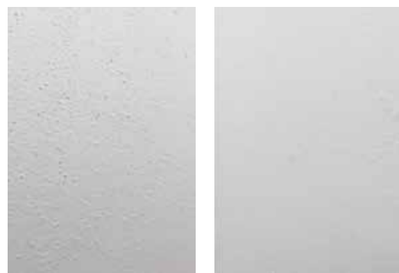
Surface defects from outgassing
