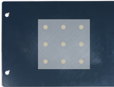
9-fold gloss measurement 60° in overlap area of the abrasion cycles.
