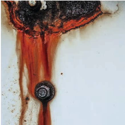
Bimetallic corrosion/galvanic corrosion
