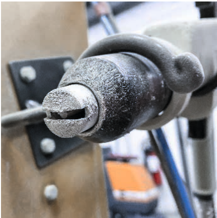
Deposits caused by sintering on the spray nozzle
