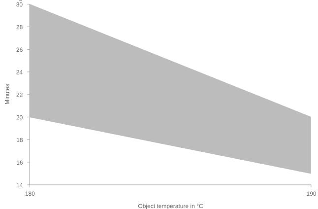
T <sub>Object</sub> t <sub>min</sub> t <sub>max</sub> 180 °C 20 minutes 30 minutes
