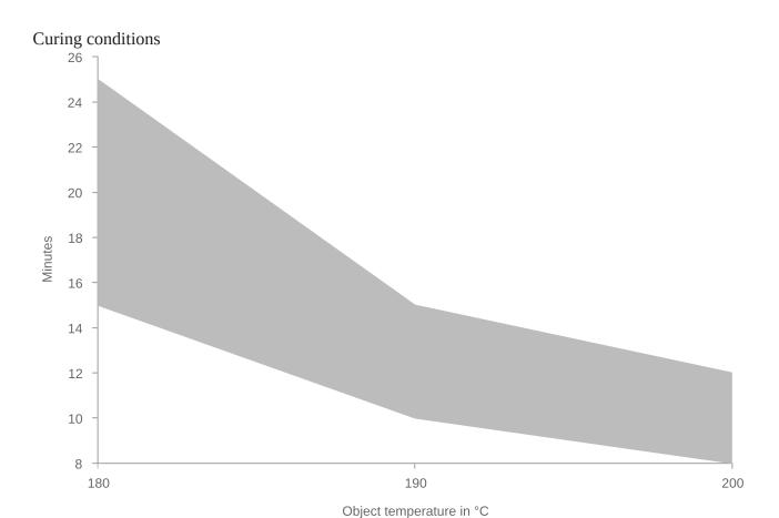
**T** Object **t** min **t** max 180 °C 15 minutes 25 minutes 190 °C 10 minutes 15 minutes 200 °C 8 minutes 12 minutes
