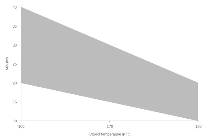
**T** Object **t** min **t** max 160 °C 20 minutes 40 minutes 170 °C 15 minutes 30 minutes 180 °C 10 minutes 20 minutes
