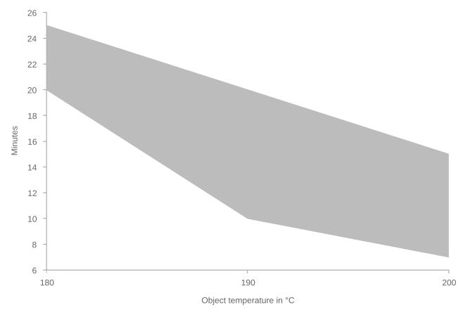
**T** Object **t** min **t** max 180 °C 20 minutes 25 minutes 190 °C 10 minutes 20 minutes 200 °C 7 minutes 15 minutes
