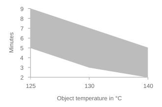
Due to the limited thermal conductivity, the use of infrared- (electric / gas catalytic) or convectional infrared combined ovens is recommended. In order to determine ideal curing conditions, we recommend practical trials with the respective object and curing oven.
