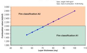
For all inorganic pigmented finished products of the IGP-DURA®mix 3302A....U00 series, a fire classification of A1 is achievable at a layer thickness of < 60µm; this is to be examined for each individual case. Organic pigmented products may vary.
