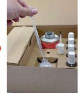
Dispense 6 ml of IGP-REPLACK curer solution into the mixing vial using a dosing pipette. The dosing pipettes have a scale of up to 3 ml.
