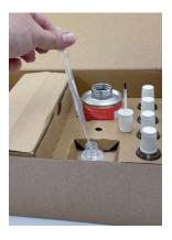
6 Dose ml of IGP REPLACK HARDENER solution into the mixing vial using a dosing pipette. The dosing pipettes have a scale of up to 3 ml.IMPORTANT:Note that when using 2 level dosing spoons of coating powder, the amount of IGP-REPLACK hardener solution must be increased to 12 ml.
