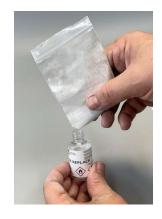
Pour the amount of powder coating filled in the ZIP bag into the mixing vial. To do this, lightly cut off a corner of the ZIP bag and let the powder coating slowly trickle into the mixing bottle through the resulting opening.
