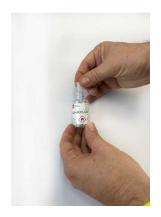
Insert a scraper insert into the opening of the mixing vial and press down firmly.
